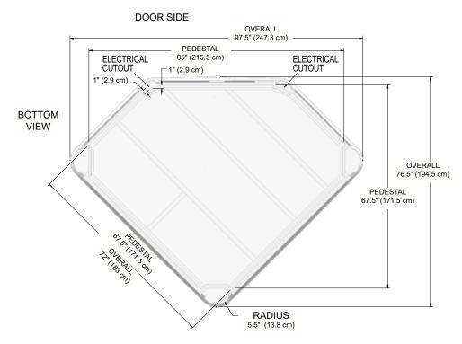
**NOTE: WATKINS WELLNESS** recommends that the TX be installed on a minimum 4" (10.2 cm) thick reinforced concrete pad or structurally sound deck able to support the "dead weight" found in the spa specification chart.
