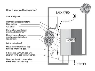
If the spa has to be taken off of the cart to go over a wall (either because the entry area is too narrow, the eaves are too low, the corner is too tight, or the stairway is too steep), a crane will be required. Don't be alarmed! About ten percent of the time, a crane is the only way to install the spa by lifting it to its final destination.
